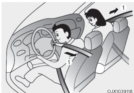
[1] : Retractor pre-tensioner seat belt Front seat and second row outboard seat (if equipped)
