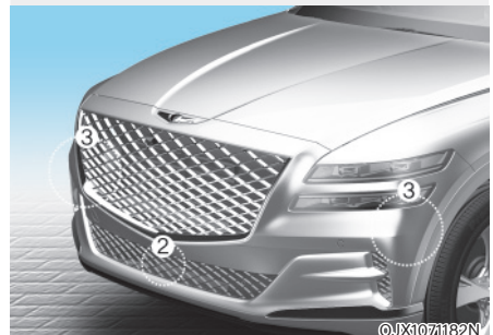
[1] : Front view camera, [2] : Front radar [3] : Front corner radar (if equipped)
