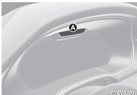
[A] : Interior view camera
