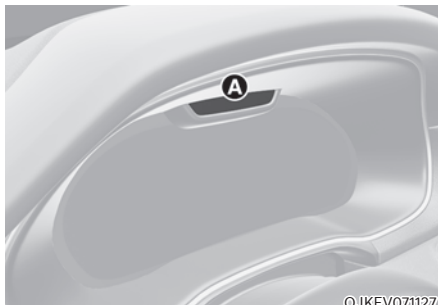
[A]: Interior view camera
