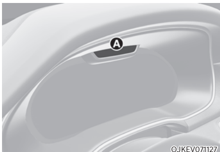
[A] : Interior view camera
