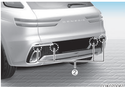
[1] : Front ultrasonic sensors, [2] : Rear ultrasonic sensors
