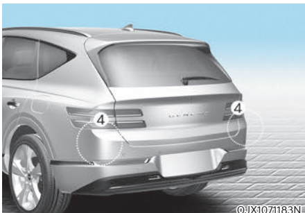
[1] : Front view camera, [2] : Front radar, [3] : Front corner radar (if equipped), [4] : Rear corner radar
