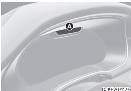
[A] : Interior view camera
