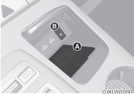
[A]: Charging pad, [B]: Indicator light
