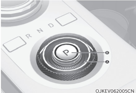
[A]: Rotary shifter (Rotary gear shift dial), [B]: P button
