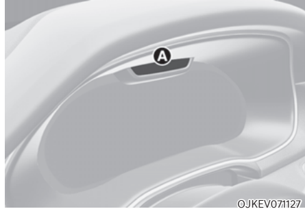
[A]: Interior view camera
