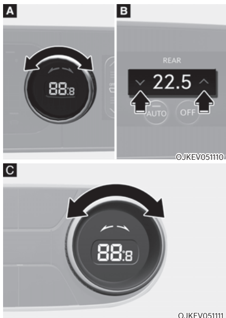
[A]: Front seat (Front seat control), [B]: Front seat (Rear seat control), [C]: Rear seat
