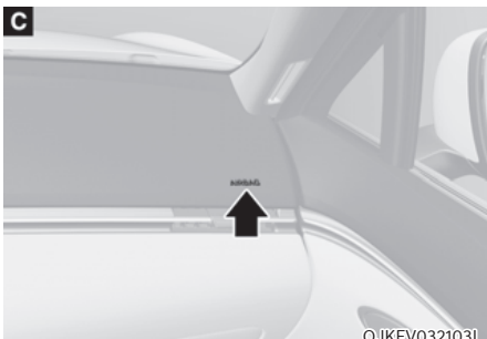
[A]: Driver's front air bag, [B]: Driver's knee air bag, [C]: Passenger's front air bag
