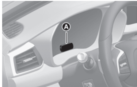
[A] Interior view camera
