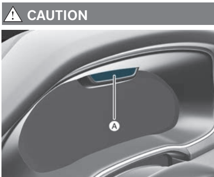
[A] : Interior view camera
