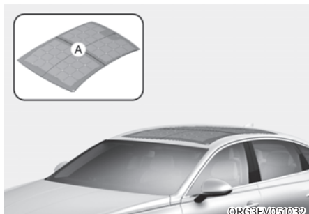
[A] : cellule photovoltaïque
